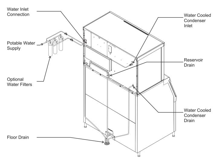
**Water Supply and Drain Connections**
